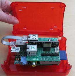
1) Carefully pull the box lid from the base using gentle rocking motion. Do not use excessive force as this may damage the box locating pins.
